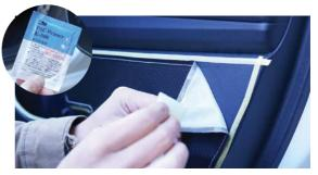
Lightly apply the 3M K500 primer on to the adhesive side of the kick panel. Firmly attach the kick panel into place.
