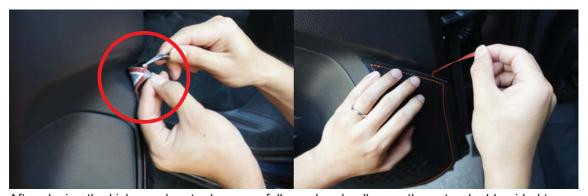
After placing the kick panel on to door, carefully peel and pull away the outer double-sided tape.
