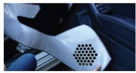
Line up and place the kick panel on to the door mounting area. Adjust the alignment if necessary.
