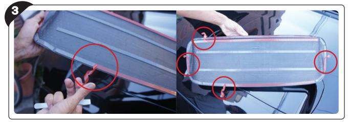
Peel a small section of film off of the tape from the sides and then fold it outward so that they can be pulled after aligning the piece into position.
