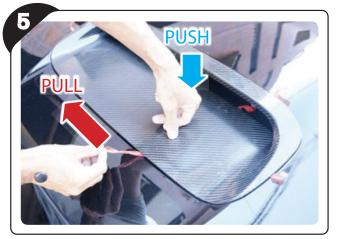
Once aligned carefully push down from the top to prevent further movement and pull out the release film to secure the carbon piece.
