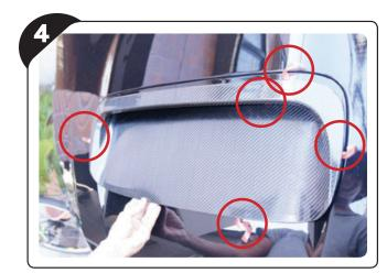
Carefully align into the desired position while making sure the red release film is on the outside of the piece.
